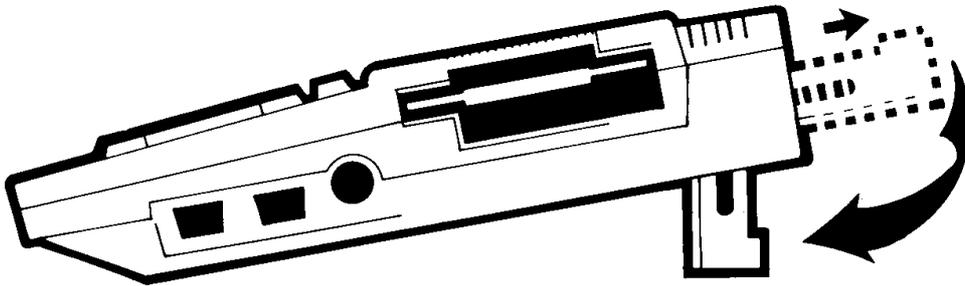
Fig. 2.1 Pulling out the Handle (Side View)
