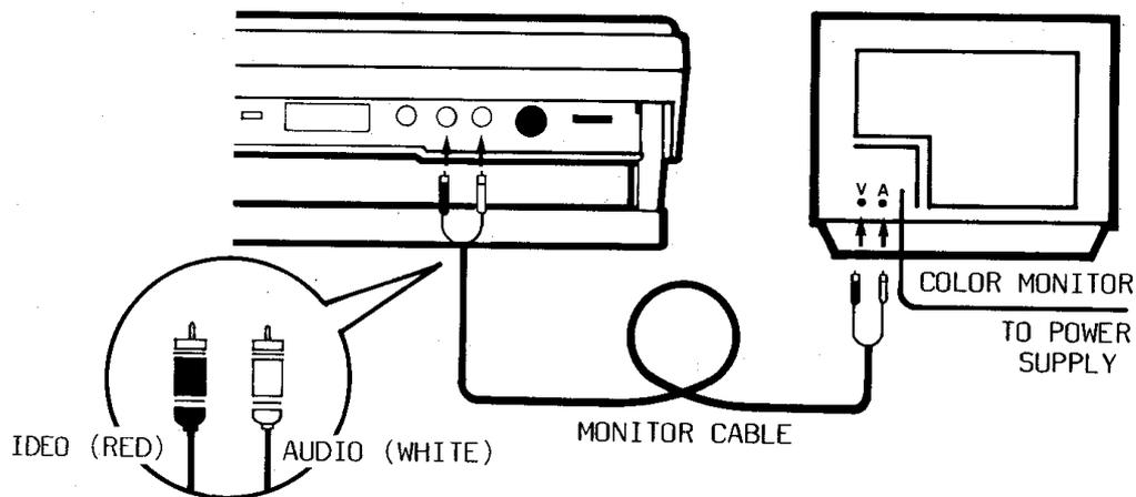
Fig. 2.5 Connecting with Monitor
