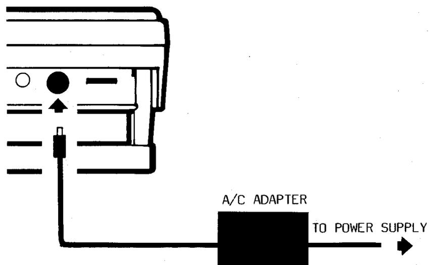
Fig. 2.9 Connecting with A/C Adaptor
