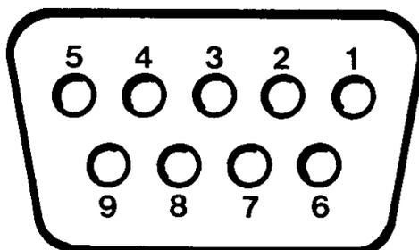
RS-232-C SOCKET PIN ASSIGNMENT (FRONT VIEW)
