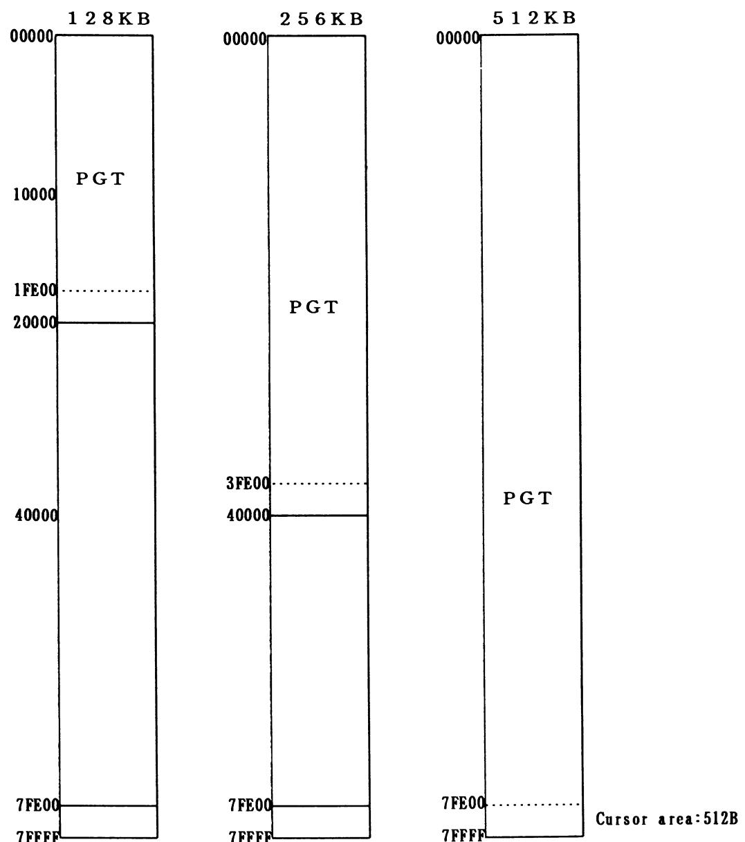
VRAM (256KB) to image space correspondence when the dot Number in the X direction of the image space is 512 at 8BIT/DOT in B1 mode.
