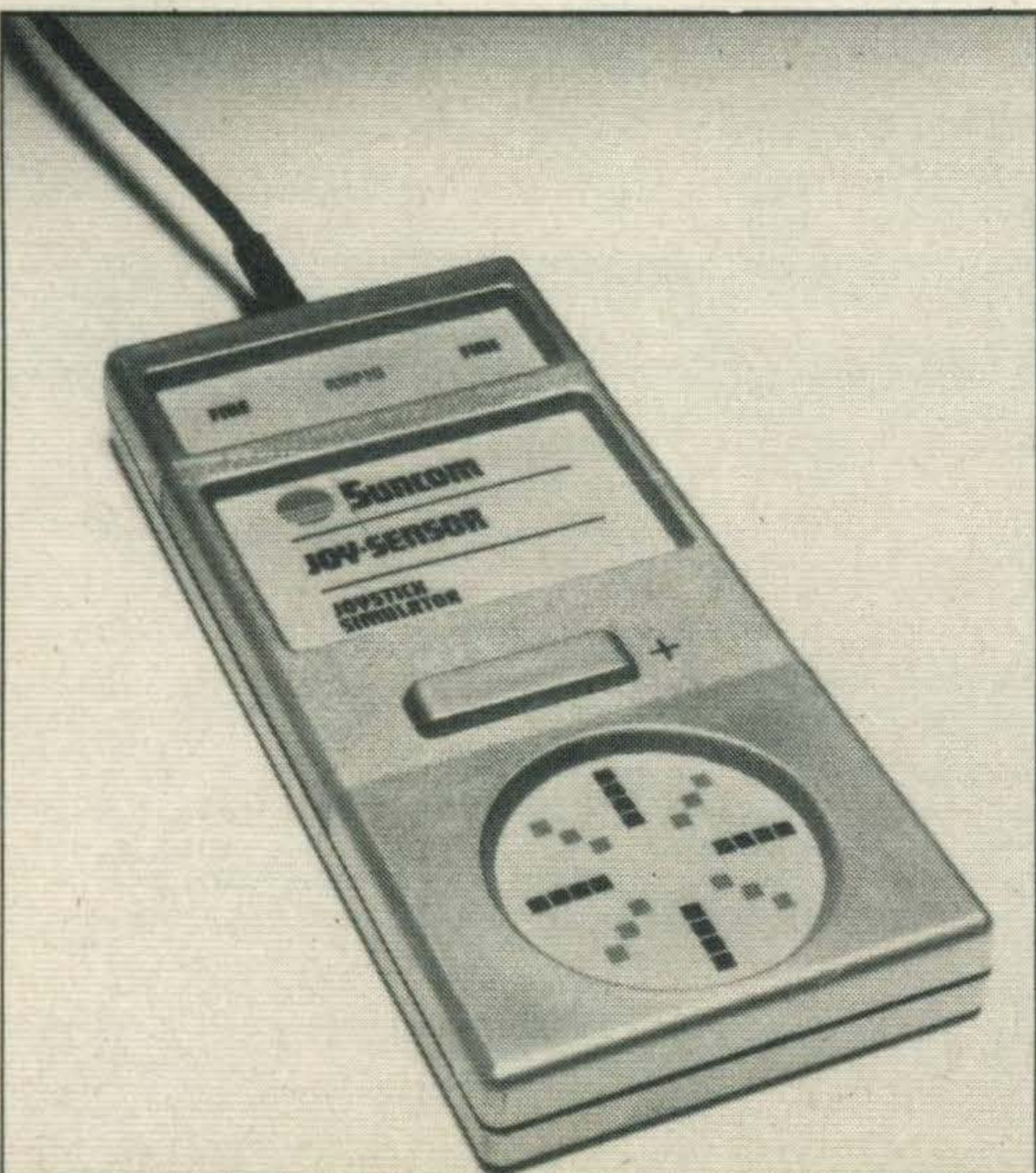
This joystick uses a touch sensitive pad
