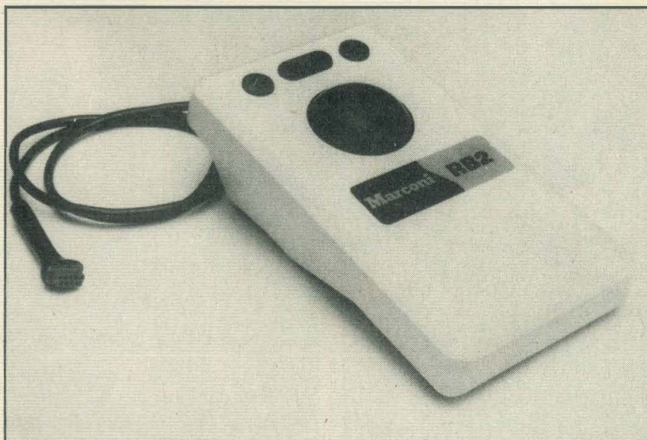
Marconi's tracker ball was developed for air traffic control systems
