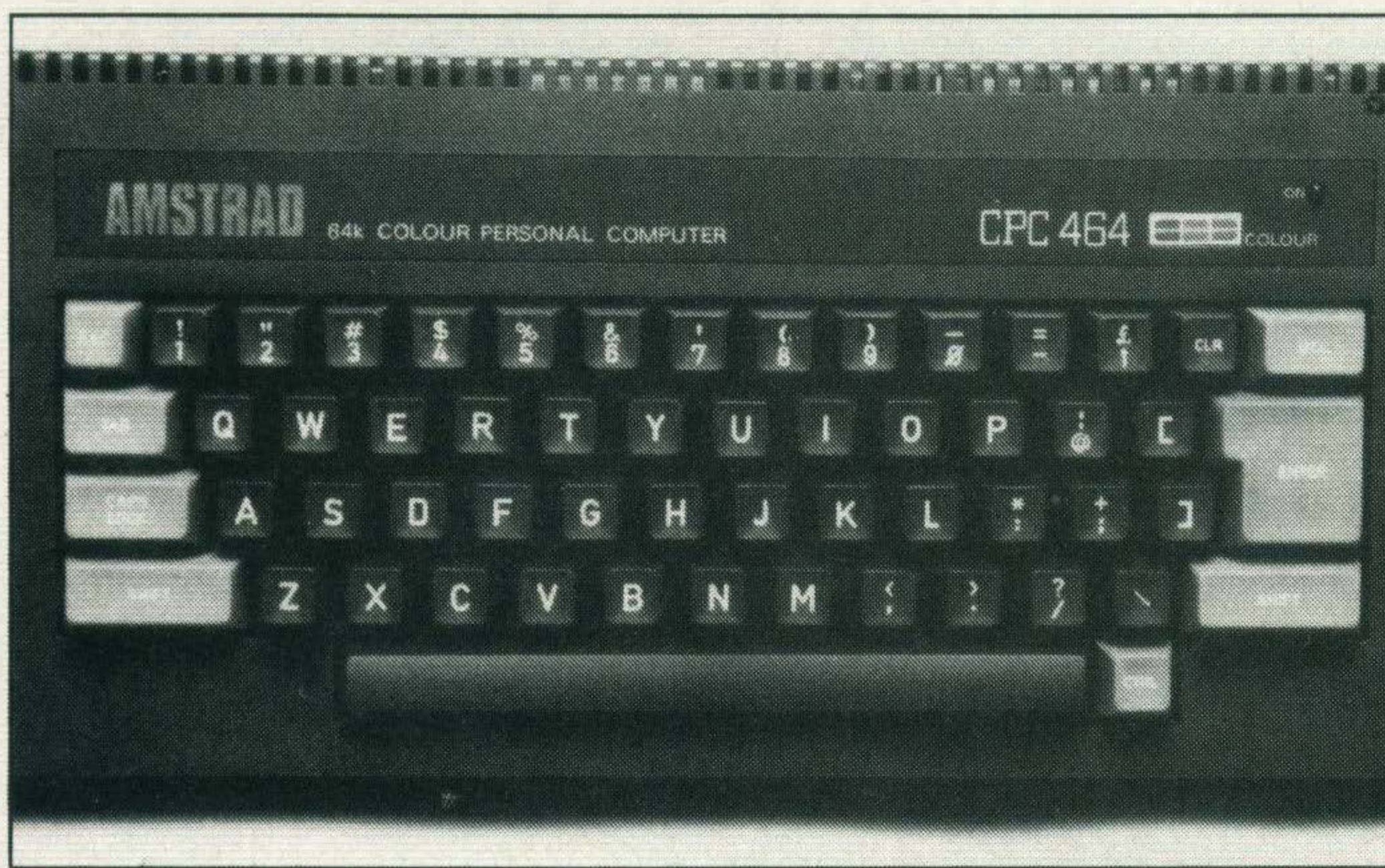
The Amstrad CPC464 keyboard is quite slim and carries an extra large ENTER Key. Unusually, it includes a numeric keypad
