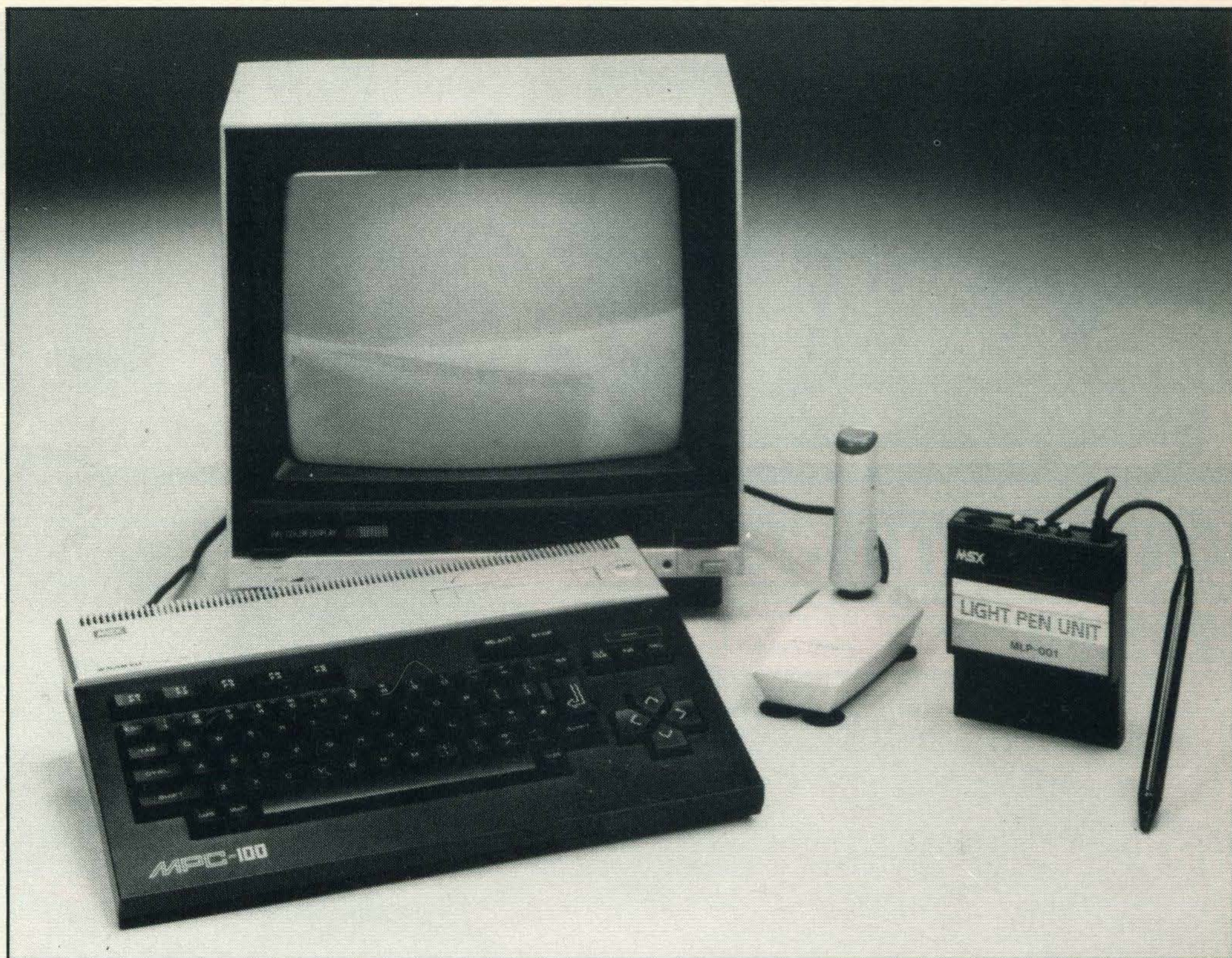
Light pen unit interfaces to the CPU through the cartridge port. Familiar MSX joystick seen here in Sanyo guise
