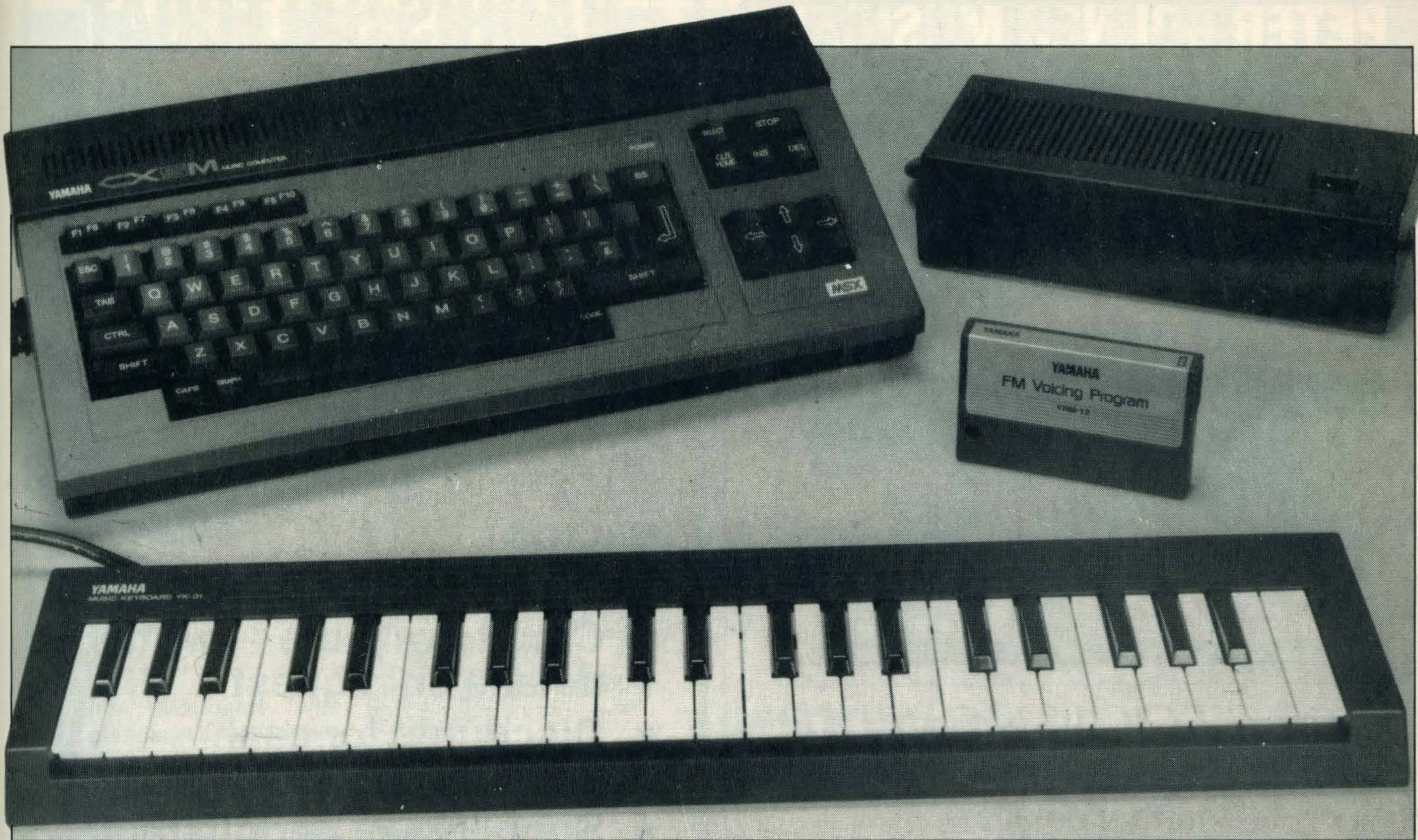
A proper piano-style keyboard is part of the £600 Yamaha CX5M outfit — more a synthesiser with an MSX computer
