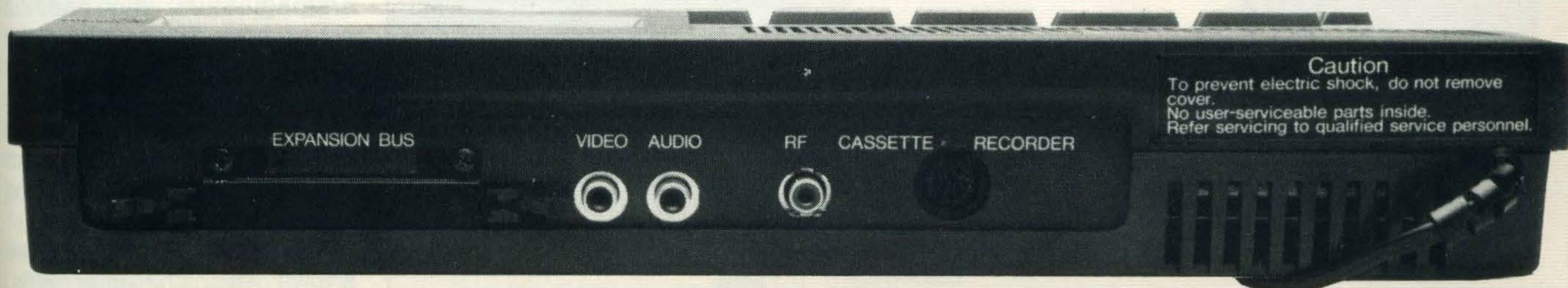
Standard MSX Input/output array but Toshiba have fitted a screw-on dust cover to their lockable 50-pin expansion bus
