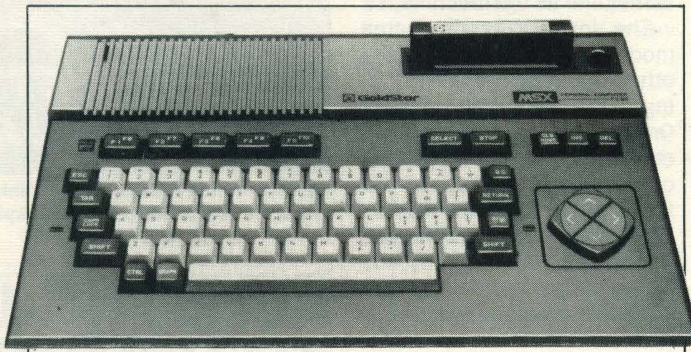
Korean Goldstar FC-80 MSX micro — a full spec machine with light pen holder and good demo program
