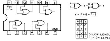
$$Y = A + B = \overline{\overline{A} \cdot \overline{B}}$$
