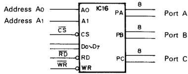
The diagram above shows the functions of 8255A. The 8255A is a programmable, general-purpose I/O device designed to construct a 8-bit microcomputer system, and it is characterized by the followings:
