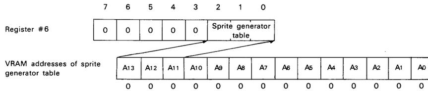
Set upper 3 bits of the head address of VRAM sprite generator table to lower 3 bits of register #6.
