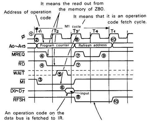
It means that the refresh address for dynamic memory is being output to address bus.
