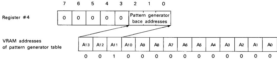
Set upper 3 bits of the head address of VRAM pattern generator table to lower 3 bits of register #4.
