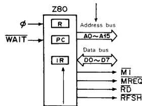
From the address of the memory, which is specified by the program counter, a part of the operation code is fetched to the command register (IR).
