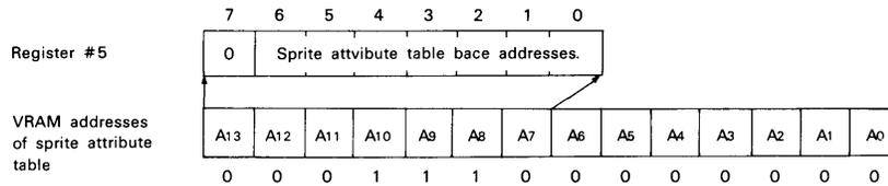
Set upper 7 bits of the head address of VRAM sprite attribution table to lower 7 bits of register #5.
