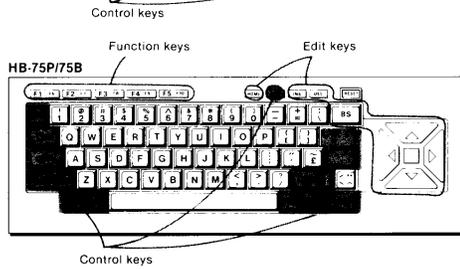
In the HB-55P, the graphic patterns are printed on the keyboard, while in the HB-75P/75B, graphic pattern decal can be affixed to the keyboard.
