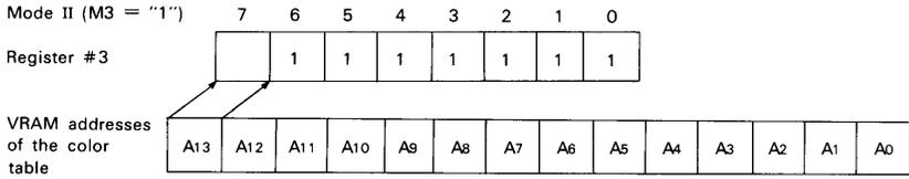
Set the uppermost bit of the head address of VRAM color table to the uppermost bit of Register #3, and set the rest of the 7 bits all to "1".
