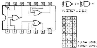
$$Y = A + B + C = \overline{\overline{A} \cdot \overline{B} \cdot \overline{C}}$$
