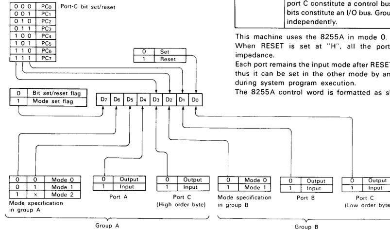
When using C port as an output port, any 1 bit only out of the 8 bits in the C port may be SET (H level)/RESET (L level) with the control word from the CPU. In this way, the program or data may be SAVED to the TAPE.
