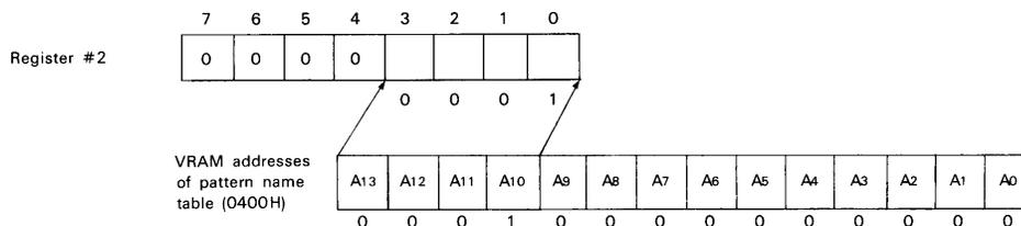
As the VRAM of VDP is up to 16K bytes (3FFFH) only and can be shown with 14 bits, the VRAM addresses become as shown in above figure.
