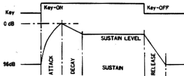
Figure III - 2 Envelope waveform
