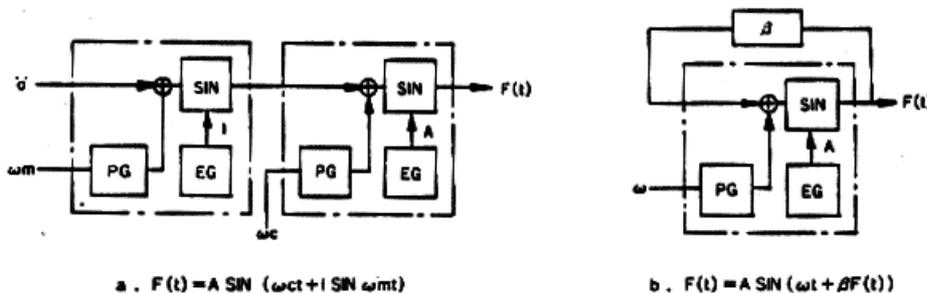
Figure I-1 Sound synthesis by FM with units
