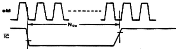
Fig. A-2 Reset Timing
