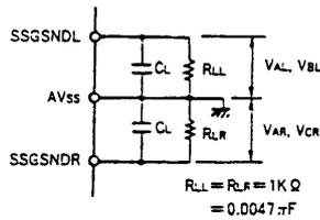
Note 9) State of registers during SSGSNDL and SSGSNDR output voltage measurement
