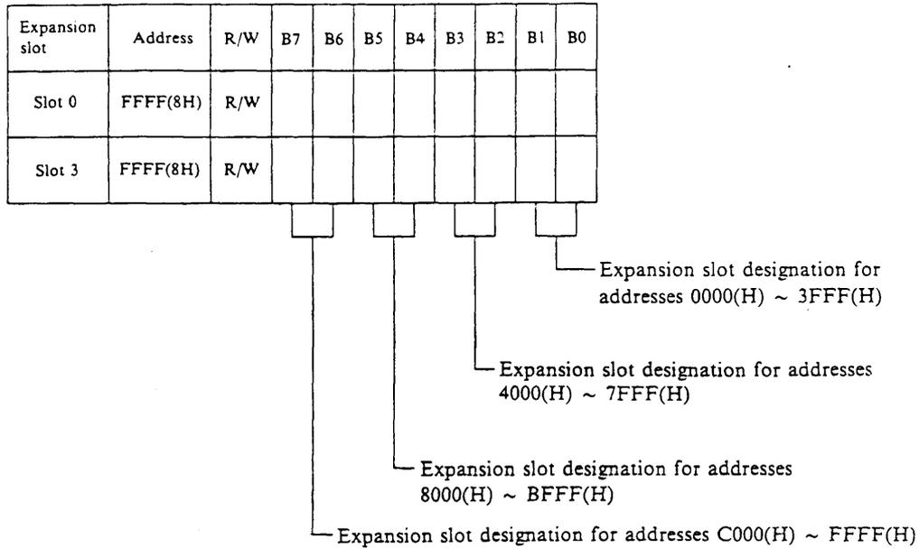
The slot expansion function is controlled by the level of the  $\overline{\text{X1}}$  and  $\overline{\text{X3}}$  pins when the device is reset. Refer to section on selection of this function.
