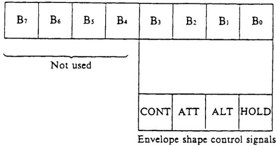
The envelope can take the shapes shown in the table below according to combinations of the CONT, ATT, ALT, and HOLD signals.
