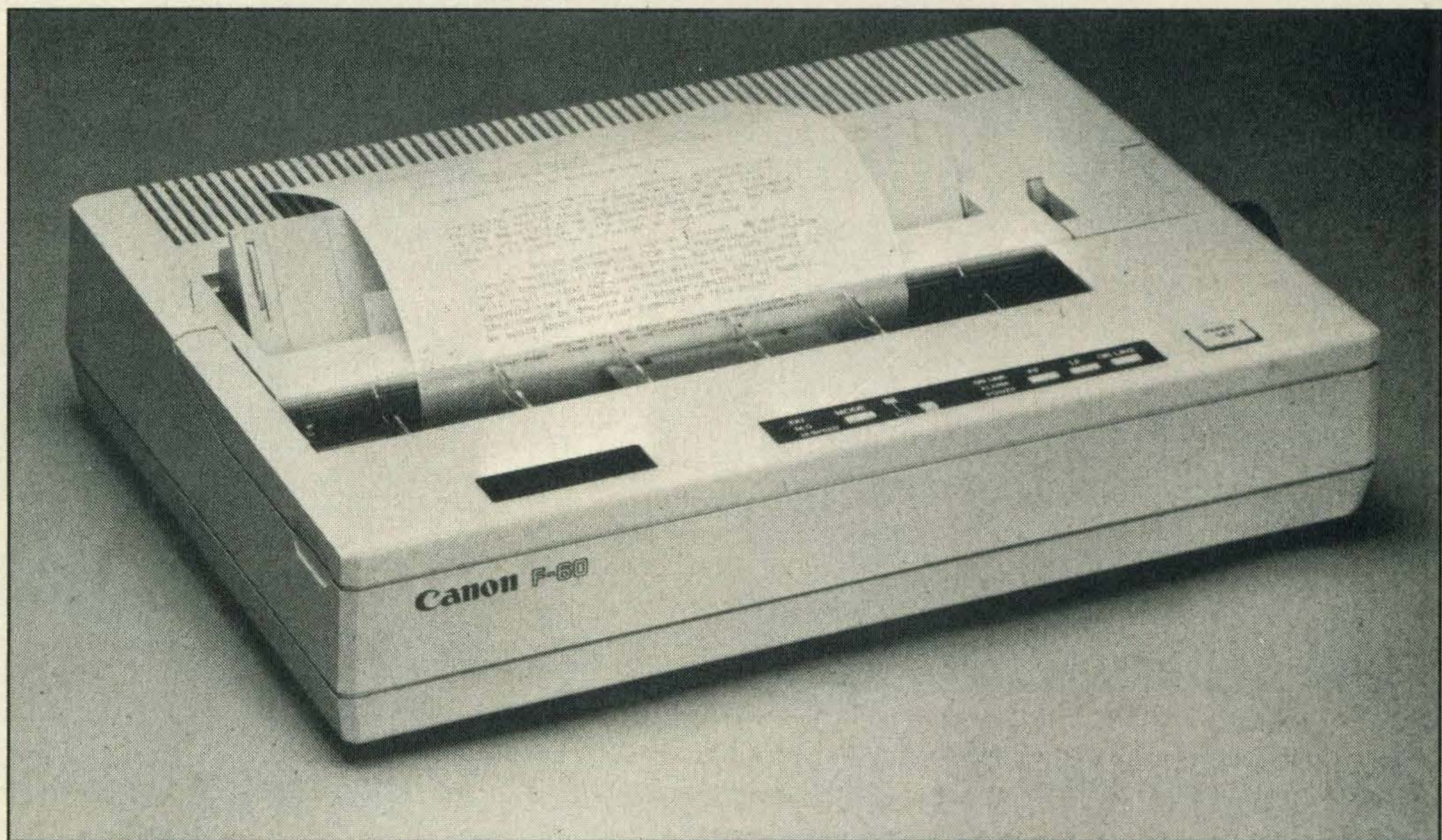
A printer is essential for business users — here's Canon's F-60 thermal dot matrix model
