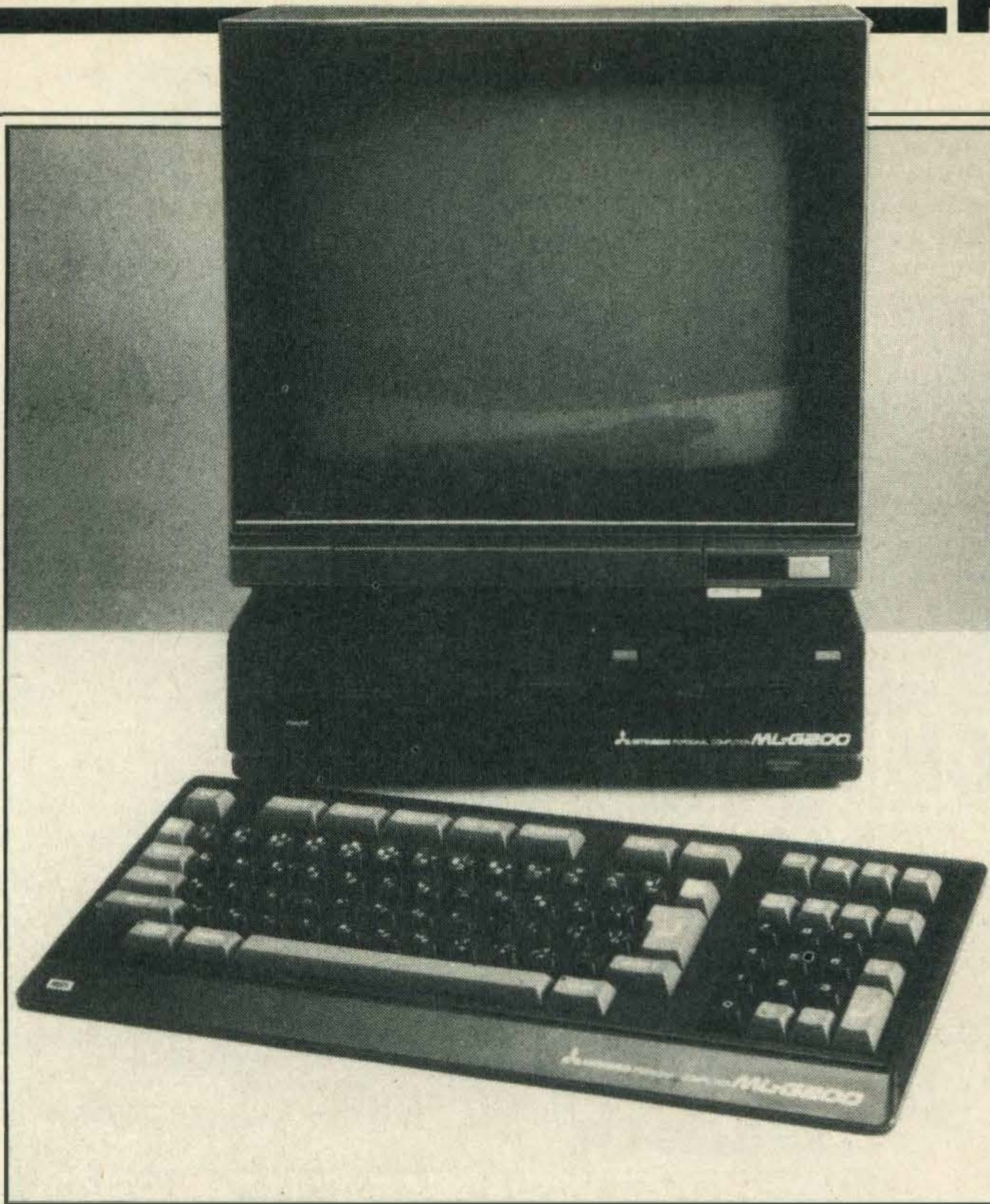
The ML-G3 comes with twin disk drives and an RS232 Interface
