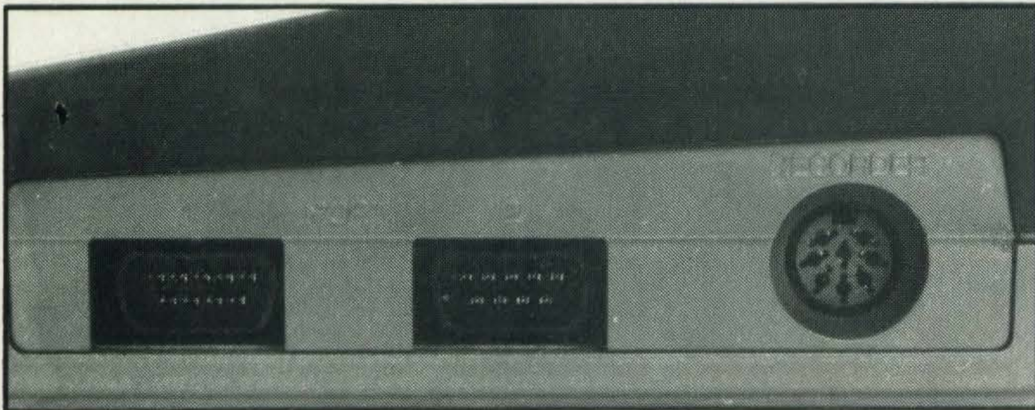
The joystick and data recorder ports ranged along the right hand side
